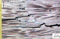
Optical micrograph showing a section through an intergranular crack in 7079-T651 (Keller's etched)
