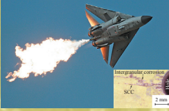
SCC service failure of 7079-T651 component from a F-111 aircraft
