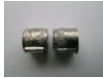
Titanium alloy compacts after sintering at high temperature in dilatometer; molybdenum support and alumina discs at each end adhering to compacts.
