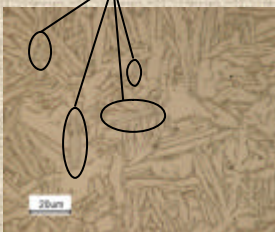
Fig. 1 - OM image of the cross section of TMC exhaust valve, showing a matrix with Widmanstätten structures
