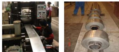
Fig. 4 Cold rolling and cold rolled coils
