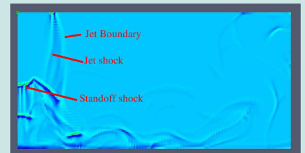
Figure 8: Round supersonic impinging jet at PR = 1.2, Ma = 2.2, s = 2 .
