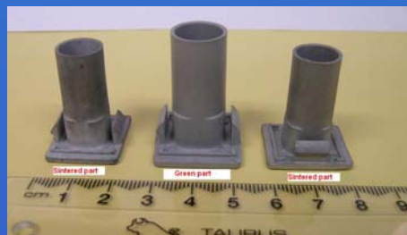
Fig.5 The metal injection moulded demonstration parts, showing that thin walled sections and distortion free complex shapes can be fabricated.
