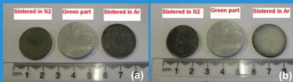
Fig. 2 Hot pressed samples of AA6061+2.0%Sn before and after sintering at 620°C for one hour in nitrogen and argon: (a) top surface (b) bottom surface. There is differential shrinkage between the top and bottom surfaces of the argon sintered sample, leading to a concave bottom surface. In contrast, the sample sintered in nitrogen is not distorted.
