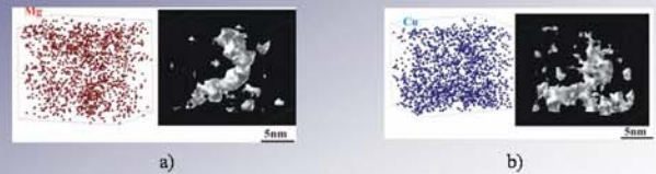
Fig. 7. a) Selected atom map and corresponding iso-concentration surface of segregation of Mg atoms on the dislocation; b) selected atom map and corresponding iso-concentration surface of segregation of Cu atoms on the dislocation.
