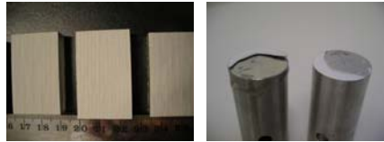
Bond strength measurements of pure Al powder KM sprayed on a pure Mg substrate
