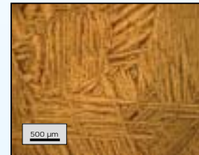
Figure 3. OM images of sintered and HIPped of pure titanium
