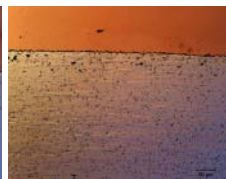
Fig.9 Optical micrograph of KM Cu coated specimen showing as-etched microstructure of Al 5005 substrate
