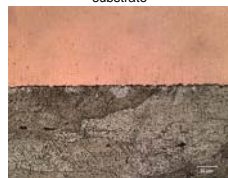
Fig.10 Optical micrograph of KM Cu coated specimen showing as-etched microstructure of Al 2124 substrate
