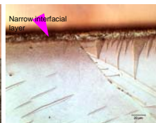
Fig.11 Optical micrograph of KM Cu coated specimen showing as-etched microstructure of CP Mg substrate
