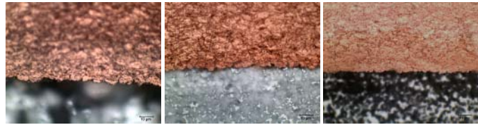
Fig.13 Optical micrographs showing as-etched microstructure of KM Cu coating on EP Al (left), Al 5005 (middle) and Al 2124 (right) substrates
