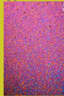
After in-situ formation of A_mC_n in the Mg-10Y melt
