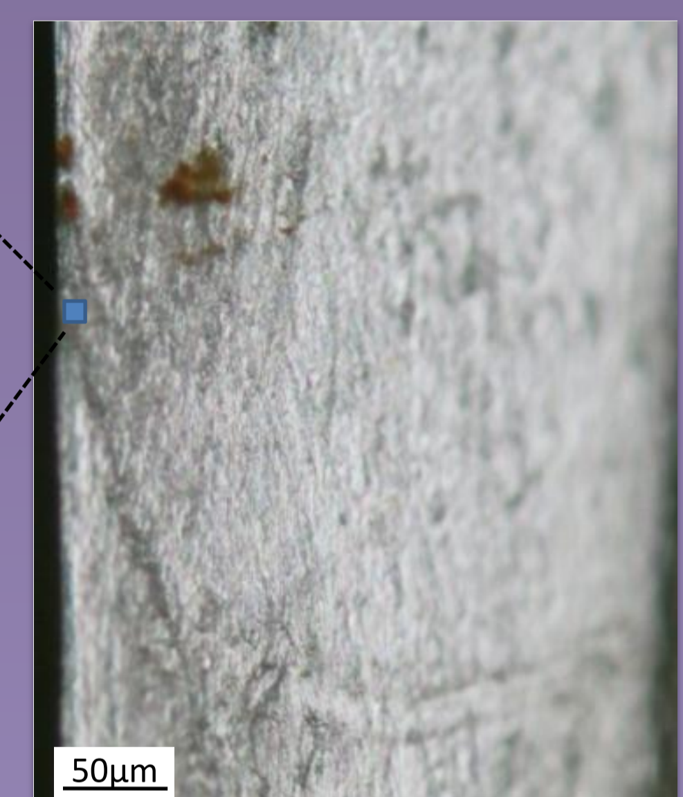
Figure 6) The deflected scratch after 1 ARB cycle.
